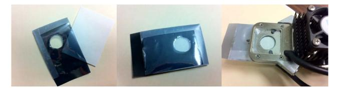
The cuvette upper and lower foam rubber gaskets must not come into contact with the filter paper once it is placed in the cuvette, as seen above, right.
