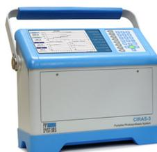
The rate of respiration of germinating seeds is easily measured using the Insect Respiration Chamber with the CIRAS-3 Portable Photosynthesis System.
