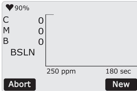
If the baseline (B) does not drop to either 0 or a very small number (typically 1-3 ppm), there is either a leak in the system, or the system has not adequately “zeroed”. Abort the process, wait 2-3 minutes, and try again. If the problem persists, inspect the injection setup for leaks and ensure that the absorber column is properly seated and contains fresh soda lime.
