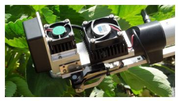
An optional, low power LED light unit is available for light control—perfect for light response curves and cloudy days. The unit clips onto the cuvette head and can easily be removed for measurement under ambient conditions.
