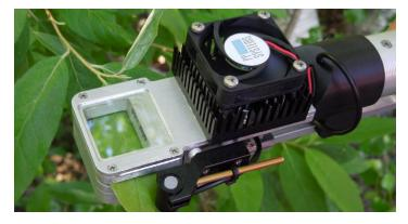
The lightweight (0.7 kg) and versatile PLC5 Leaf Cuvette is ideal for a wide variety of vegetation including broad leaves, narrow leaves, grasses and small needle conifers, and includes sensors for measurement of air temperature and PAR. All leaf cuvette materials are carefully selected to minimize influences such as infrared radiation, water sorption,  $\mathrm{CO}_2$  effects and leaks. The leaf gaskets provide an air-tight seal without causing damage to vegetation.
