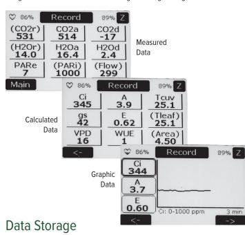
Data storage is virtually unlimited. Data is stored on a USB flash drive (memory stick) for safe storage and easy transfer of data to your PC.
