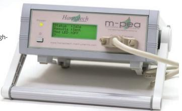
The system is controlled from a comprehensive Windows® software package (M-PEA+) which allows complex experiments to be designed, uploaded and executed by the M-PEA hardware. Recorded data is quickly downloaded to the software via a USB 2.0 connection.
