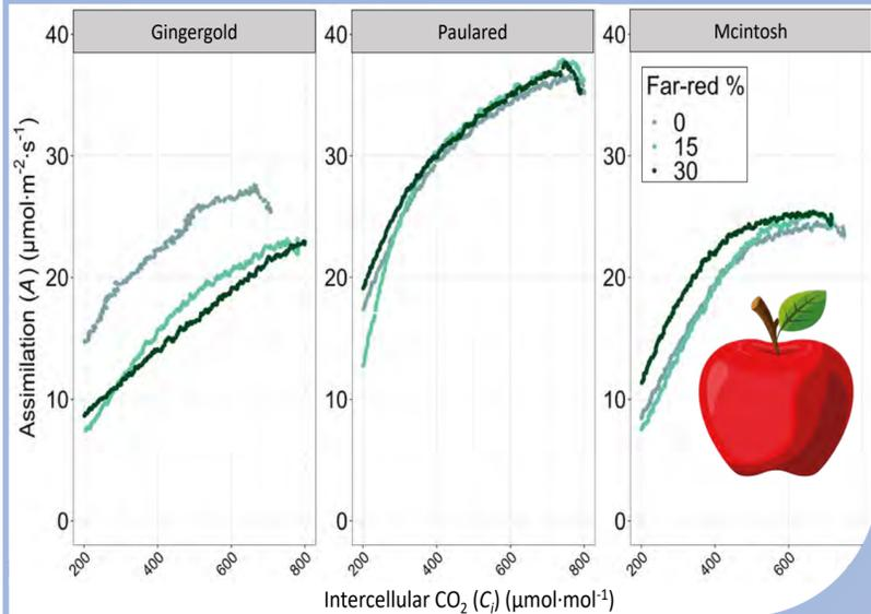
**Figure 3:** A vs. C<sub>i</sub> curves for three cultivars of Apples in the open-field. CO<sub>2</sub> was ramped upward from 200 to 1000 μmol·mol<sup>-1</sup> at a rate of 150 μmol·mol<sup>-1</sup>·min<sup>-1</sup> using the SSCO<sub>2</sub>R™ method.
